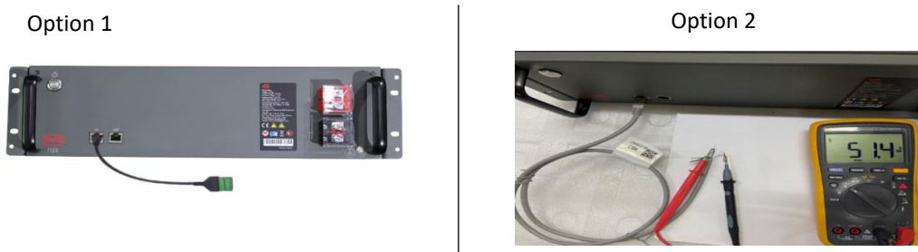
Figure 5 voltage measurement on pin 7&8
